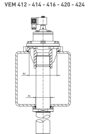
**Note:** Fix the valve body to the tank using the appropriate eyelets in the valve body
